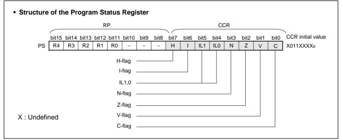
The RP indicates the address of the register bank currently in use. The relationship between the pointer contents and the actual address is based on the conversion rule illustrated below.
